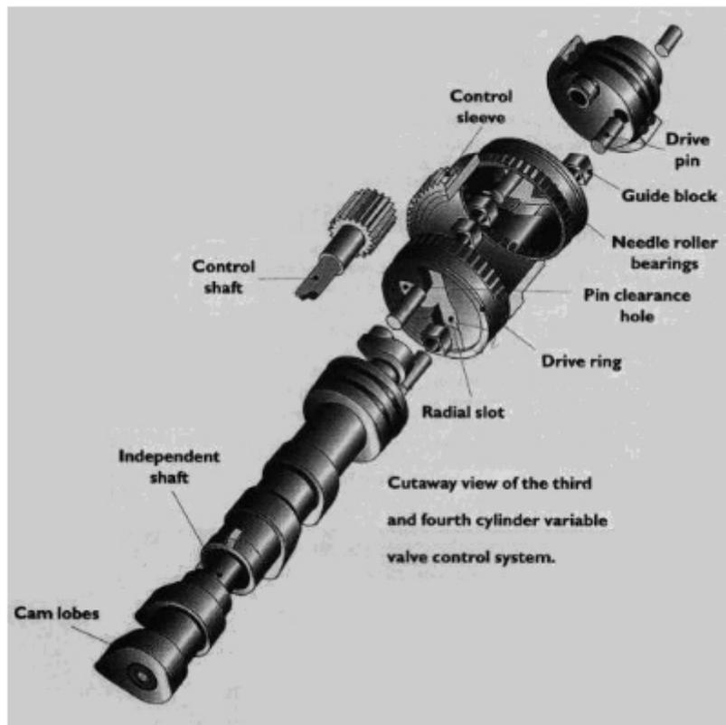
The really ingenious bit is the design of the VVC Mechanism. As the cross-sectional diagrams show, the outer control sleeve is machined such that it is much thinner on one side than the other, (i.e. its bore is eccentric to its outside diameter). The sleeve can be adjusted through about a quarter-turn which causes the pair of drive rings within the sleeve to move outside the camshaft's centre of rotation.
