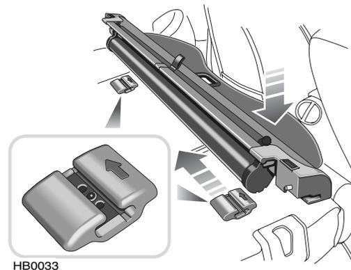
1. Detach the safety net/loadspace cover cassette from its normal position behind the rear seats.
