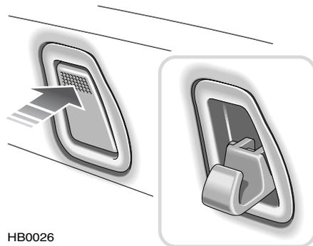
On some cars, two retractable carrying hooks are set into the side trim panels in the loadspace. Use these to secure bags or loose items, which might, otherwise, move around the loadspace in response to the car's momentum.
