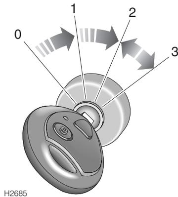
The starter switch is located to the right of the steering column and uses the following sequence of key positions to operate the steering lock, electrical circuits and starter motor:
