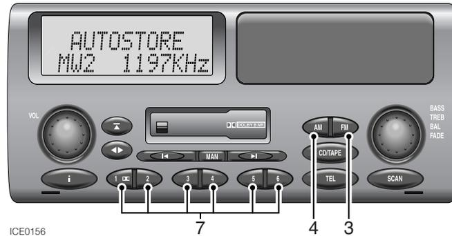
Auto-store enables you to rapidly tune and store the strongest FM and MW radio signals in a single operation. This facility is particularly useful if you are in an unfamiliar area and have little knowledge of local transmitter frequencies.
