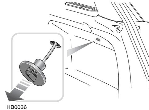
If, for any reason, the fuel filler flap automatic unlocking mechanism fails, the flap can be released manually by pulling a release cord in the loadspace area.
