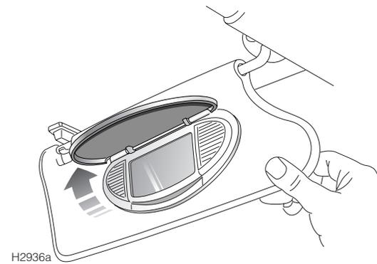
Pivot the sun visor downward to use the vanity mirror. On some models, the vanity mirror has a cover and is illuminated when the cover is raised. Close the cover to extinguish the lights.
