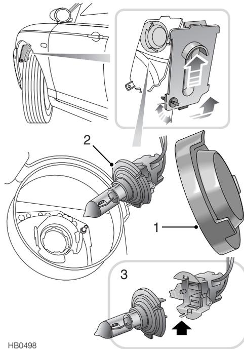
Turn the front wheels to full left or right lock. This provides room to reach into the wheel arch to remove the headlight access panel.
