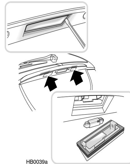
To access a bulb, use a small flat-bladed screwdriver to ease the lens from the underside of the applique (see upper inset - the lever action of the screwdriver will compress the spring retaining clip and enable the lens to be pulled free). Prise the connectors apart to remove the bulb.
