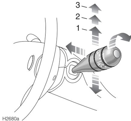
The wipers and washers will only operate when the starter switch is in the first or second position.
