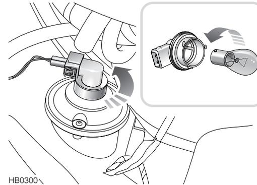
Detach the electrical connector from the rear of the bulb holder by squeezing the clips on both sides of the connector and pulling the connector away from the light unit.
