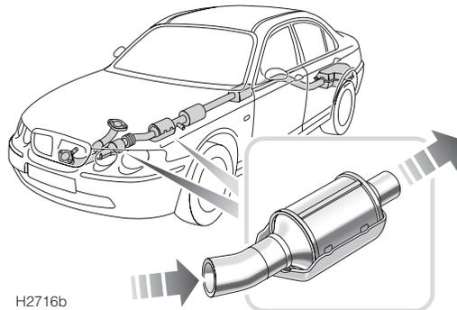
The exhaust system incorporates one or two catalytic converters, which convert poisonous exhaust emissions from the engine into environmentally less harmful gases.
