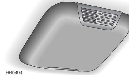
Interior space protection (ultrasonics) is designed to protect the interior of the car from intrusion (entry by a thief through a smashed window, for example). Ultrasonic sensors, mounted on the roof lining, monitor the interior space and activate the alarm if air movement is detected in the passenger compartment.
