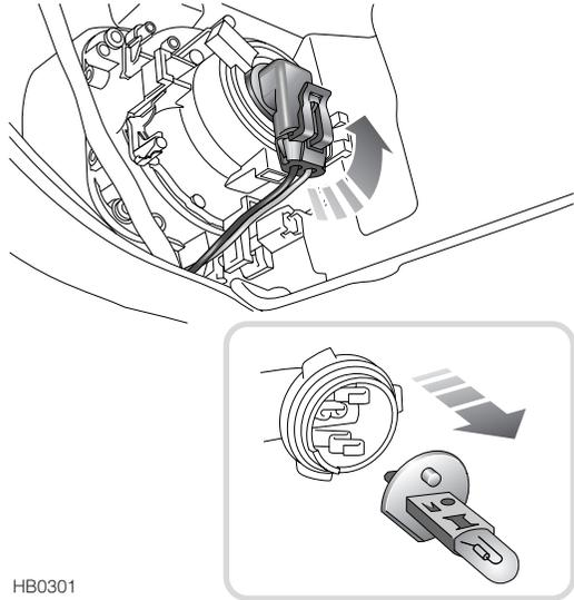
Detach the electrical connector from the rear of the light unit by lifting the lever on the side of the connector and pulling the connector downward. Twist the bulb holder an eighth of a turn
