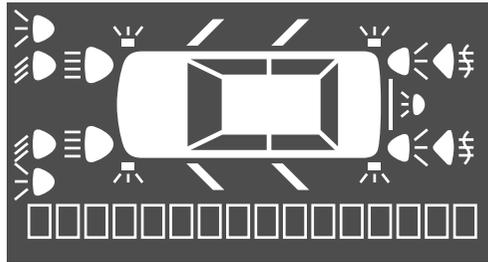
On instrument packs that incorporate a message centre, information concerning various aspects of the car's status is displayed by a combination of icons and words in the display at the upper centre of the instrument panel.
