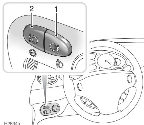
**NOTE:** *Both the rear and front fog lights are switched off automatically when the main lighting switch or the starter switch are turned off, and will need to be reselected when the starter switch is turned back on.*
