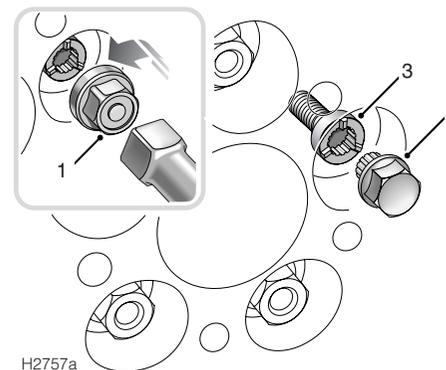
Cars with alloy wheels are fitted with one locking wheel bolt to each wheel. These are similar to standard wheel bolts, but have a removable cap (1) and can only be removed using the special adaptor (2) provided in the tool kit.
