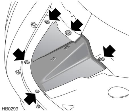
To access the light unit, the small panel immediately below the relevant light must be removed from the underside of the car. This is held in place by five Philips type screws, which must be removed before the panel can be released (see illustration for location of the five screws).
