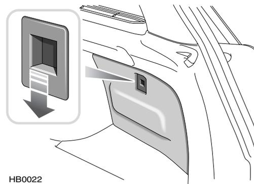
Some cars are equipped with enclosed storage compartments, one on each side of the loadspace. To remove a storage compartment cover, pull the catch down (see inset). When replacing, ensure the catch is pushed up fully to secure the cover in position.
