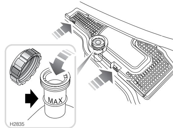
Remove the detachable mesh panel on the driver's side of the car to access the brake fluid reservoir. The fluid level can be seen through the reservoir neck and should be maintained as close to the 'MAX' mark as possible. **DO NOT** allow the level to drop below the 'MIN' mark.
