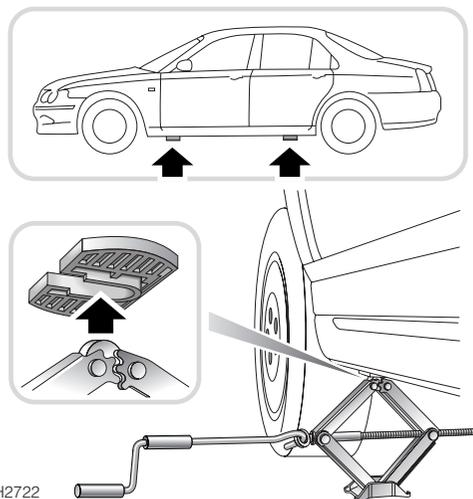
Position the jack on firm level ground under the jacking point nearest the wheel to be removed. Note that the domed head of the jack must fit into the corresponding recess in the sill plate (see inset in illustration).
