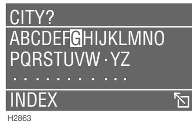
Highlight and select 'CITY?', then use the typewriter menu to enter the town or city name. Once the name is entered, the bar at the bottom of the display highlights 'INDEX' or 'ENTER', depending on the following:
