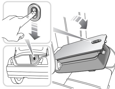
A fold down hatch is fitted in the middle of the rear seat. This enables longer loads to be carried at the same time as two rear passengers.
