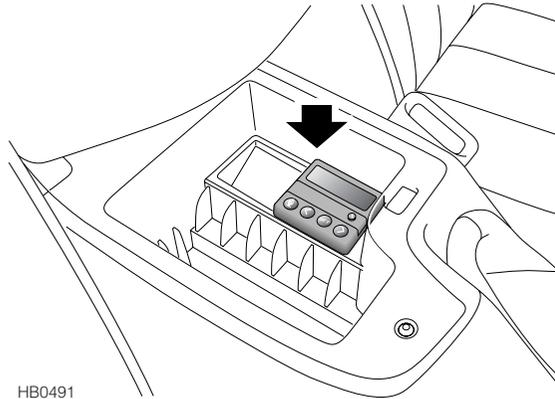
The parking heater timer unit is located in the centre console cubby box. Up to three separate preset operating start times can be programmed, each running for a maximum of 30 minutes.
