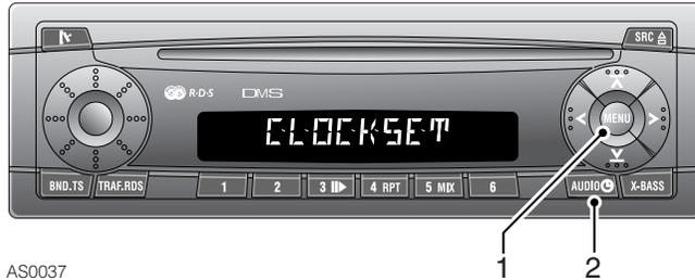
To display the time, press and hold the clock control (2). The display will be present for approximately two seconds.
