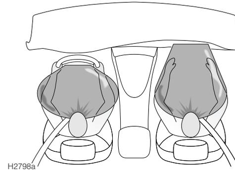
Airbag inflation is virtually instantaneous and occurs with considerable force, accompanied by a loud noise. The inflated bag, together with the seat belt restraint system, limit the movement of a front seat occupant, thereby reducing the risk of injury to the head and upper torso.
