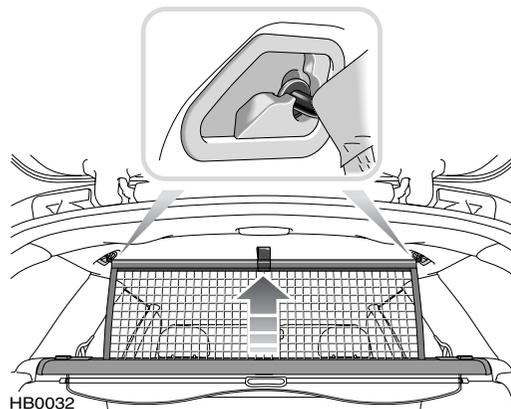
On some cars, the loadspace cover cassette also incorporates a safety net, designed to prevent loose loads and items of luggage from encroaching into the passenger compartment in the event of an accident or emergency manoeuvre.
