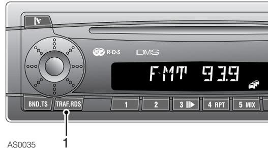
On the FM waveband, your radio is able to receive traffic information broadcasts automatically as and when they occur.
