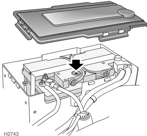
To access the battery, unclip and remove the battery cover as shown in illustration.
