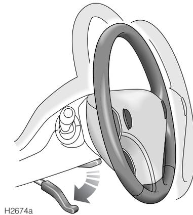
Adjust the angle and height of the steering column to suit your driving position:
