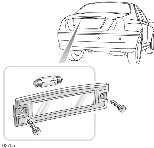
There are two number plate lights. On saloon models, remove the two securing screws and the lens to access each bulb.
