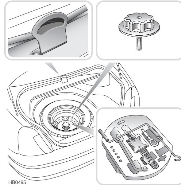
Raise the carpeted floor panel, using the lifting handle (set into the floor) and hook the handle over the boot drain channel.
