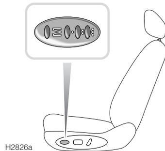
Your car can memorise three different driver seating positions. To store the positions in the system memory, the starter switch must be turned to the first or second position.
