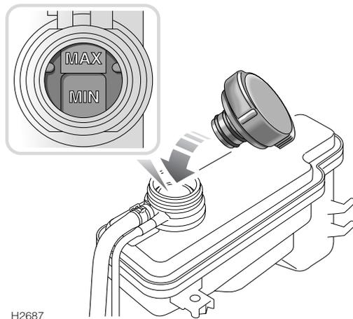
Remove the filler cap to check the level of the coolant. The level marking can only be viewed through the filler neck.
