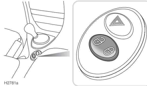
This is a personal security feature which allows the driver to lock (or unlock) all the doors from inside the car (while driving or with the car stationary). Press the closed padlock symbol on the switch to lock (the alarm will not be armed), and the open padlock symbol to unlock.
