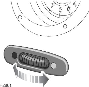
Air supply from the face level vents is further controlled by the heater bypass control in the centre of the fascia panel.
