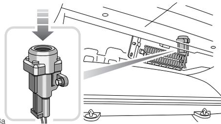
In the event of a collision or sudden impact, an inertia switch automatically cuts off the fuel supply to the engine and, providing the alarm is disarmed, unlocks the doors.
