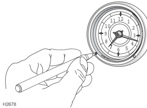
To adjust the clock, use a ball point pen or similar probe to advance or retard the hands, by pressing the right or left hand buttons at the bottom of the clock bezel.
