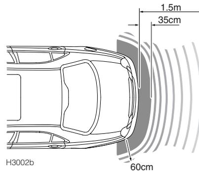
Four ultrasonic sensors, situated in the rear bumper, scan an area behind the car searching for obstructions. If an obstruction is detected, the sensors calculate its distance from the rear of the car and communicate this information to the driver by sounding warning chimes. It is important to remember that the system is no more than an AID to parking. It is not foolproof in operation, nor is it a substitute for observation and personal judgement.
