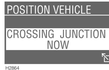
Repeat the above procedure to enter the name of the road where you are currently situated. The navigation computer asks you to enter a 'JUNCTION'. This is the name of the road that you will next come to. Select 'JUNCTION', then enter the name using the typewriter (if required), or select the correct road name if a list of names is displayed. 'CROSSING JUNCTION NOW' appears in the display, requesting you to press the select menu control as you cross the junction.
