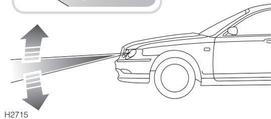
Using the following load conditions as a guide, adjust the headlights by rotating the adjuster wheel (see inset):
