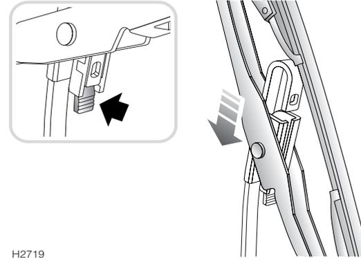
Lift the wiper arm away from the windscreen and set the blade at 90° to the arm as shown. Disconnect the blade by pushing in the locking tab (arrowed in inset), setting the blade at 45° to the arm and sliding the blade down the arm.
