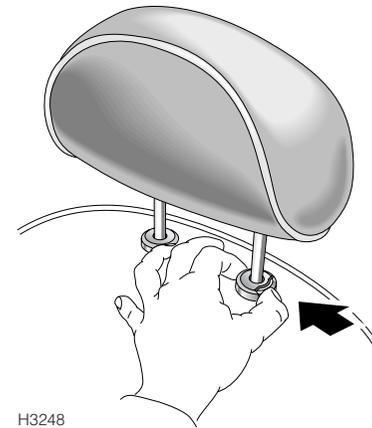
Raise or lower the restraint until the cushion is level with the back of the head.
